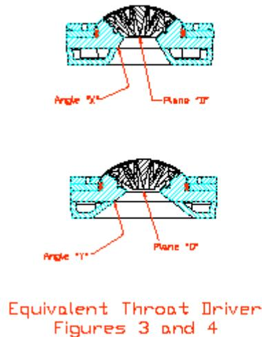
It can be seen in Figure 3 that angle "x" begins at plane "D". Because this angle begins at plane "D" the driver/horn combination provided directional control to the wavefront at the optimal point, where the radius is smallest and the high frequency limit bandwidth is greatest. Figure 4 is the same driver but shows angle "y" beginning at plane "D". It is typical for a horn with a rectangular radiation pattern (i.e. 90 degrees horizontal by 40
