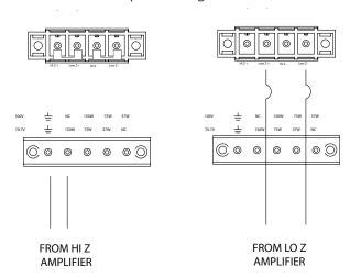
"NOTE: There are four shorting links installed on the 4 position barrier strip. Two are used in each position and are "stacked" in parallel. ALL four shorting links must be removed for Low Z operation. ALL four shorting links (two in each position) MUST be used for Hi Z (70Vrms or 100Vrms) operation." Full wiring instructions for Hi Z and Low Z operation are found on the last page of the product data sheet.
